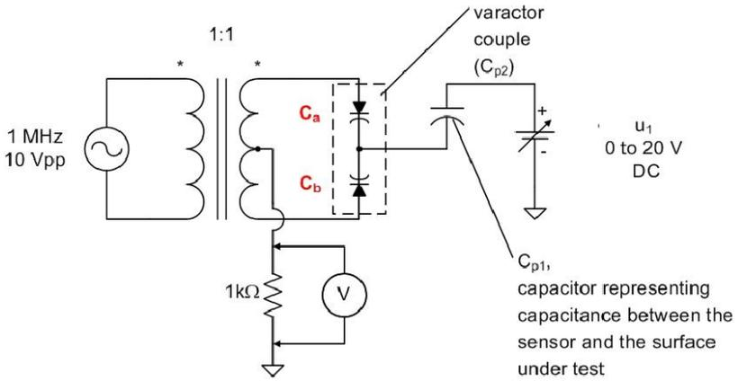
Figure 2. Varactor-based variable capacitance [12]
