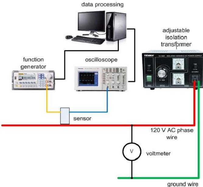
Figure 3. Test setup
