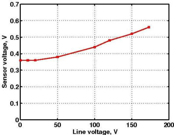
Figure 4. Example result of the AC voltage sensing
