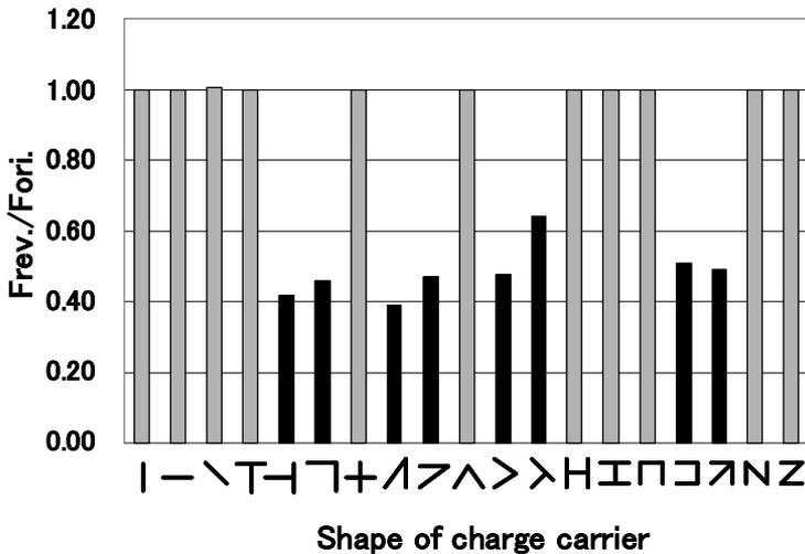
Fig. 10. The ratio of the force of reversed field to the force of original field that was calculated from the improved simulation result.
