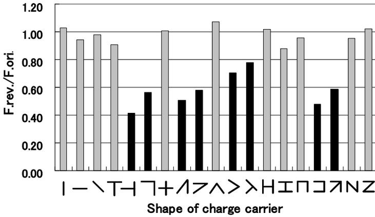
Fig. 6. The ratio of the force of reversed field to the force of original field that was calculated from experimental measured shift distance of the 19 different shape charged conductors.
