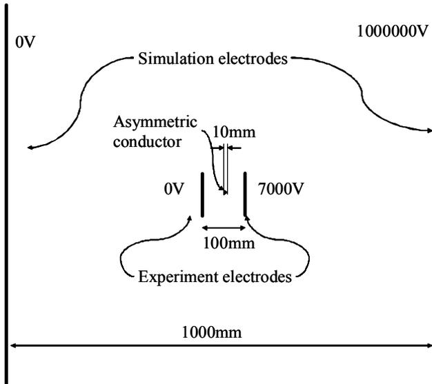
Fig. 8. Layout of electrodes of the simulation and the experiment.
