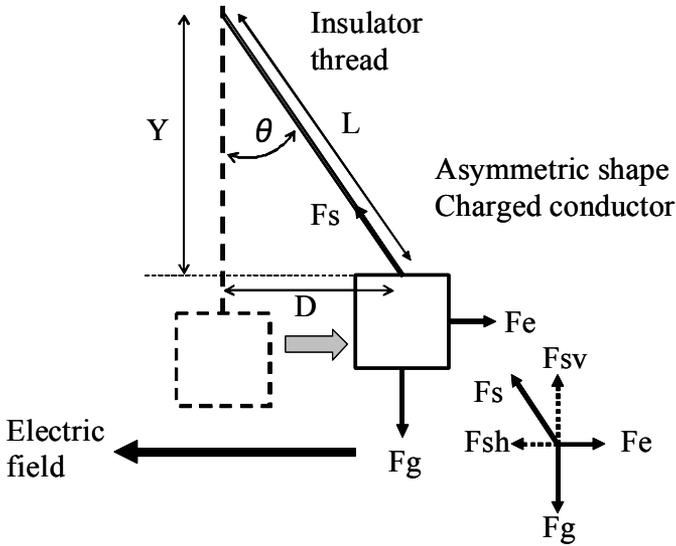
Fig. 5. Schematic diagram of the electrostatic force, the gravity force and the tensile force that act on the charged conductor in a high electric field.
