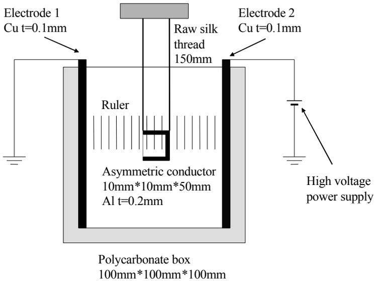
Fig. 3. The front view of the experimental instrument
