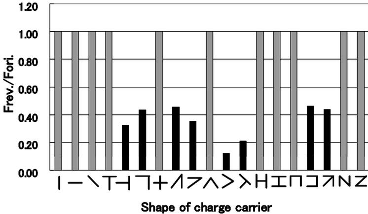
Fig. 2. The ratio of the force of reversed field to the force of original field. Both forces act on the 19 different shape charged conductors.
