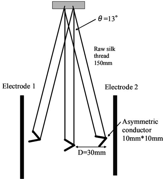
Fig. 9. Three positions and its inclines of an asymmetric conductor.
