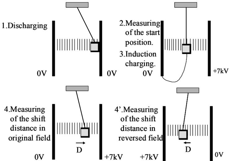
Fig. 4. A schematic of the experimental procedure
