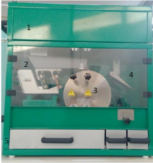
Fig. 3. Photography of the tribo-electrostatic roll-type separator : 1. Tribo-charging device; 2. Vibratory electromagnetic feeder; 3. Grounded electrode; 4. High-voltage electrode; 5. Three-compartment collector.
