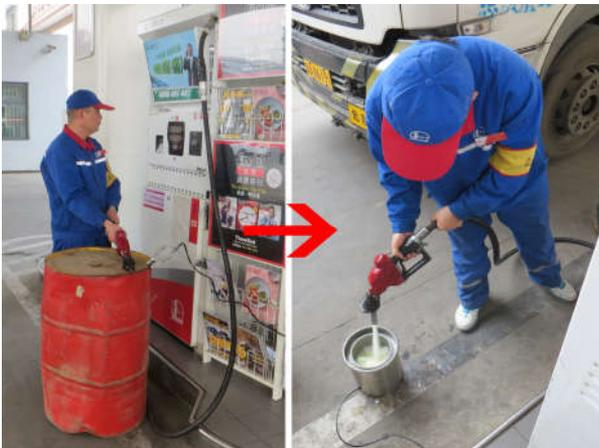
Fig.2 Pictures of measuring the level of charge accumulation during refueling in China
