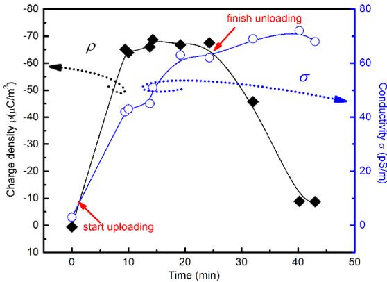
Fig.3 Change in charge density and diesel conductivity during the simultaneous uploading and refueling process in China's Shaanxi province
