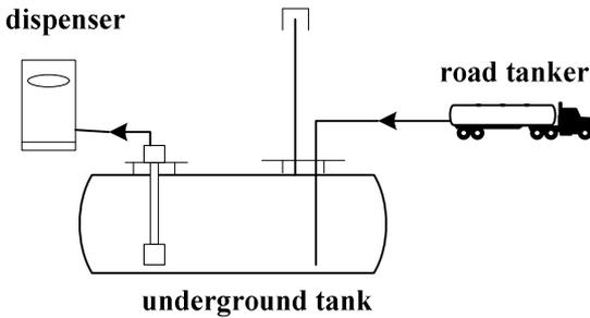
Fig.1 Schematic of a typical petrol station
