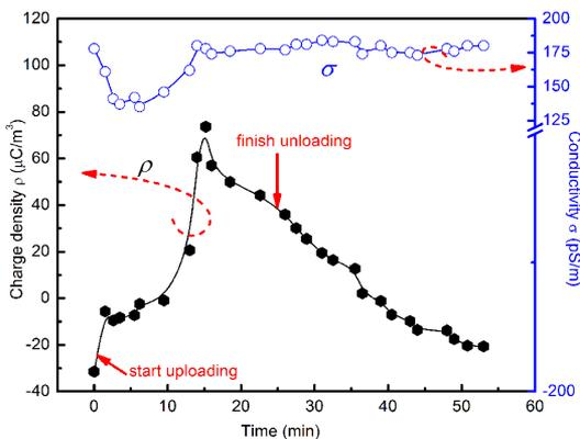
Fig.4 Change in charge density and gasoline conductivity during the simultaneous uploading and refueling process in Beijing
