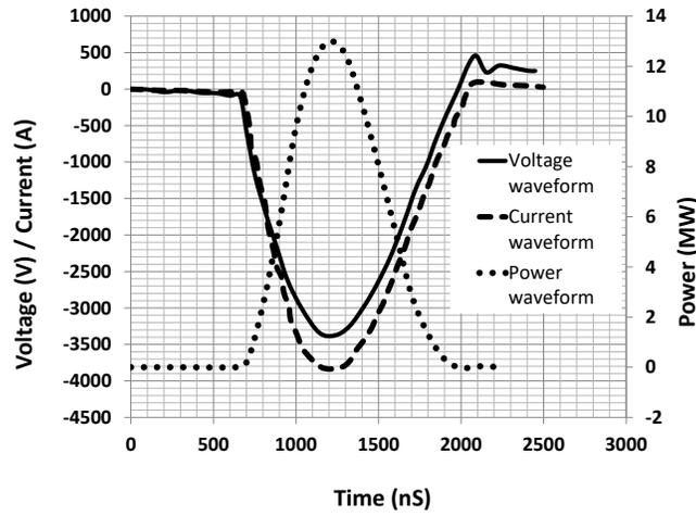
Fig. 1. Typical voltage and current waveforms generated during PEF treatment of beer
