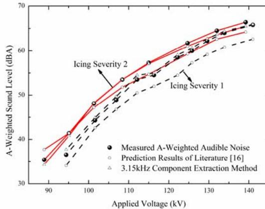
Fig. 4. Comparison of the measured A-weighted audible noise, the proposed 3.15 kHz component extraction method and 8 kHz prediction method of literature [16] under different icing severities
