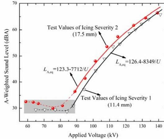
Fig. 1. Influence of icing severity on A-weighted energy-equivalent sound level of soft rime ice-covered conductor (values in shaded area are not critical)
