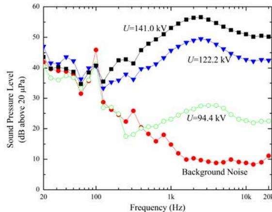
Fig. 2. The 1/3 octave spectrum of background noise and three different corona intensities of soft rime ice-covered conductor under icing severity 1
