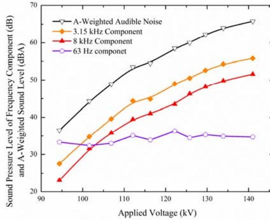
Fig. 3. A-weighted AN and characteristic 1/3 octave frequency components versus applied voltage under icing severity 1
