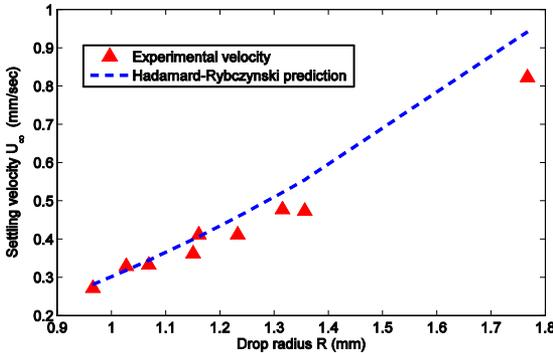
Fig. 2. Plot showing the variation of the settling velocity with drop radius for a drop falling under the influence of gravity alone. The experimental data (in red) has been compared to theoretical results (in blue)
