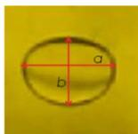
Fig. 5. Drop deformation is quantified in terms of the deformation ratio which depends on the lengths of the polar and equatorial axes of the drop.
