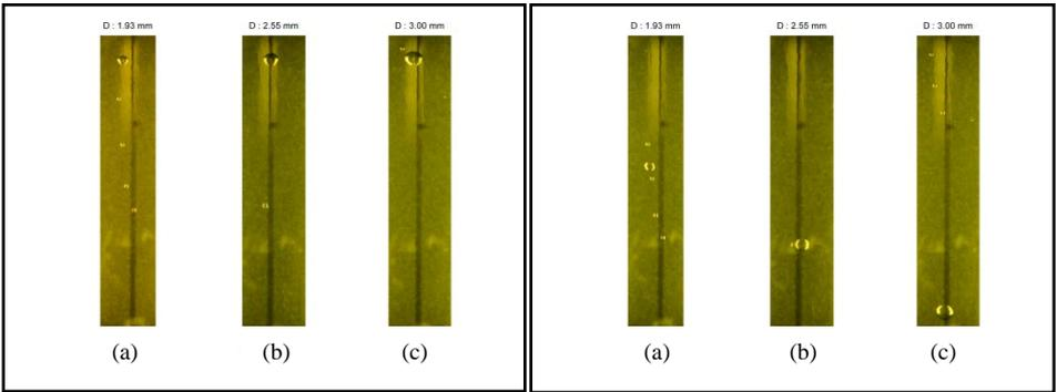
Fig. 3. Variation of settling velocity with drop speed. The image on the left shows the position of three drops of different sizes at  $t=0$ . The image on the right shows the positions of the same drops at  $t=68$  sec. The applied electric field is  $3.33$  kV/cm.
