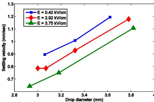
Fig. 4. Variation of drop settling velocity with drop diameter for different electric fields
