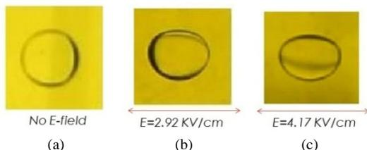
Fig. 6. Drop shape observed by increasing the electric field from 0 to 4.17 kV/cm (peak value). The drop diameter is similar in all the three cases.
