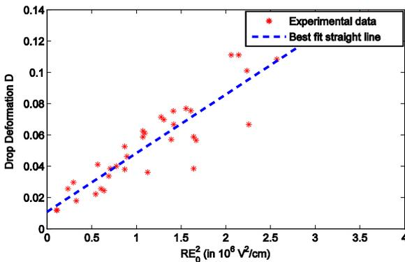
Fig. 7. Plot showing variation of drop deformation with  $E_0^2 R$
