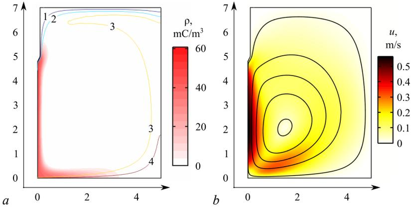
Fig. 2. (a) Surface plot of space charge density distribution and contour plot of relative temperature (1—0.2, 2—0.4, 3—0.6, and 4—0.8  $\Delta T$ ), and (b) surface plot of fluid velocity and flow streamlines in an injection EHDHE at  $\sigma_0 = 10^{-11} \text{ S/m}$ .
