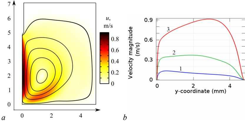
Fig. 5. Contour plot of fluid velocity and flow streamlines at  $\sigma_0 = 10^{-9}$  S/m (a) and axial velocity distributions for three values of the conductivity ( $1-10^{-10}$ ,  $2-3 \cdot 10^{-10}$ , and  $3-10^{-9}$  S/m) in an EHDHE based on the Wien effect.
