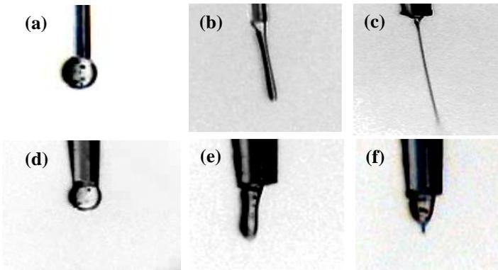
Fig.5: Electrospun jet behavior of different polymer solutions: (a) RTV615 without external electric field; (b) RTV615, using the conventional system; (c) RTV615, using the charge modifier and ethanol as a surrounding solvent; (d) SA without external electric field; (e) SA, using the conventional system; (f) SA, using the charge modifier and water as a surrounding solvent.
