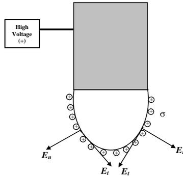
Fig. 1: Representation of tangential and normal electric fields at the fluid surface with the application of high voltage.
