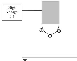
Fig. 3: Representation of the presence of surface charge at the fluid surface of an insulating liquid.
