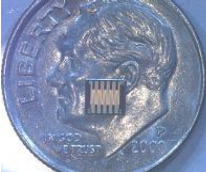
Figure 1: Top down optical image of a >1\text{kW} power MEMS switch on a dime
