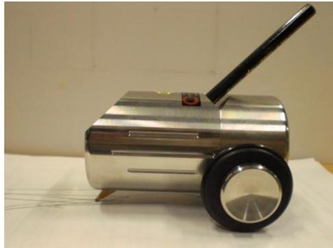
Fig. 3. Pencil hardness tester.
