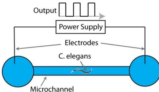
Fig. 1. Schematic of the experimental setup. Worms were loaded individually into the channel, pneumatic flows were eliminated, a desired pulse DC signal was applied and the worm response was recorded in a video format. The videos were then analyzed for speed and turning time measurements
