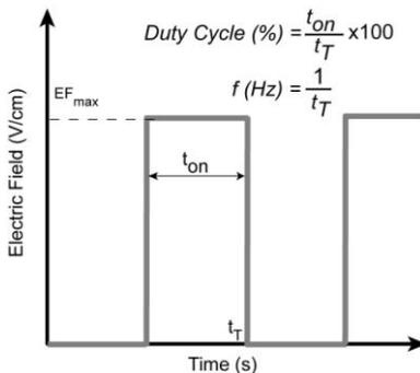
Fig. 2. Pulse DC electric field signal wave-shape.  $EF_{\text{max}}=3$  V/cm in all experiments. Effect of frequency and duty cycle on forward motion speed and turning time was studied.
