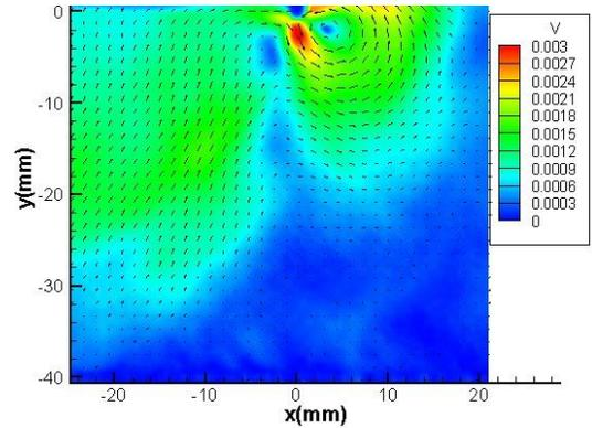
Fig. 4a. Color map of velocity modulus (m/s) and velocity vectors in the  $xy$  plane for a 5kV EHD jet,  $H=4$ cm
