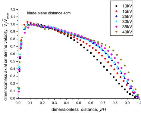
Fig. 5. Centerline velocity evolution of the EHD jet for various applied potentials with 4cm blade-plane distance
