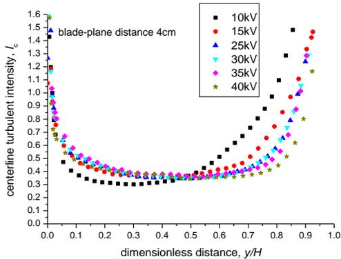
Fig. 7. Streamwise evolutions of turbulent intensity for different potential with 4cm blade-plane distance
