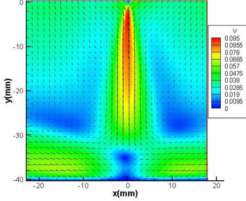
Fig. 4c. Color map of velocity modulus (m/s) and velocity vectors in the  $xy$  plane for a 40kV EHD jet,  $H=4\text{cm}$
