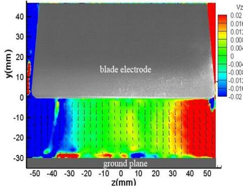
Fig. 3. Color map  $V_z$  (m/s) and velocity vectors in the  $yz$  plane for  $x=0$
