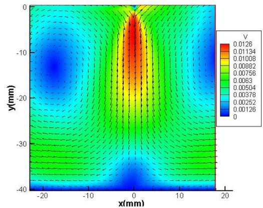
Fig. 4b. Color map of velocity modulus (m/s) and velocity vectors in the  $xy$  plane for a 10kV EHD jet,  $H=4$ cm
