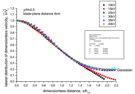
Fig. 6. Non-dimensionalized velocity profiles distribution of  $\bar{V}/V_c$  for various applied voltages at position  $y/H=0.5$  with 4cm gap
