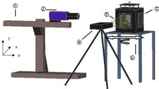
Fig. 1. Experimental facility: (1)-displacement systems; (2)-CCD digital camera; (3)-experimental cell;(4)-double pulse Nd:YAG laser; (5)-laser sheet; (6)-supporter platform
