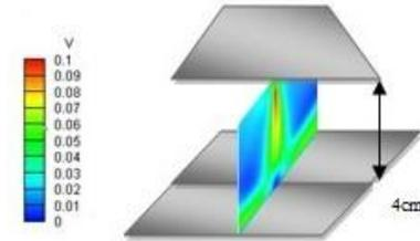
Fig. 2b. xy plane for the PIV measurement
