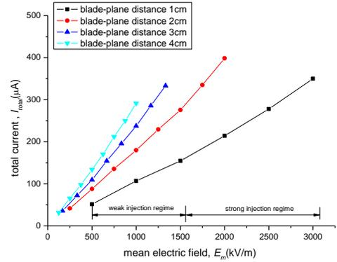
Fig. 8. Evolution of the total current versus mean electric field for different distance.
