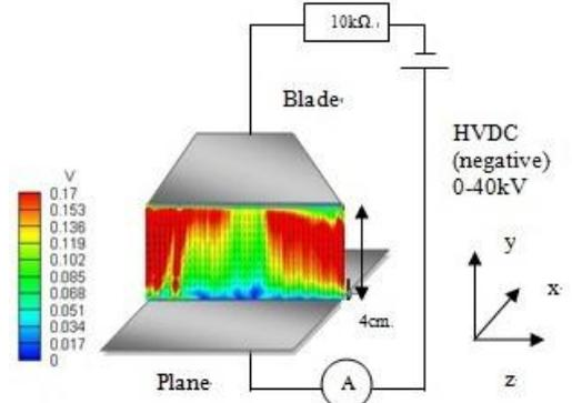
Fig. 2a. yz plane for the PIV measurement
