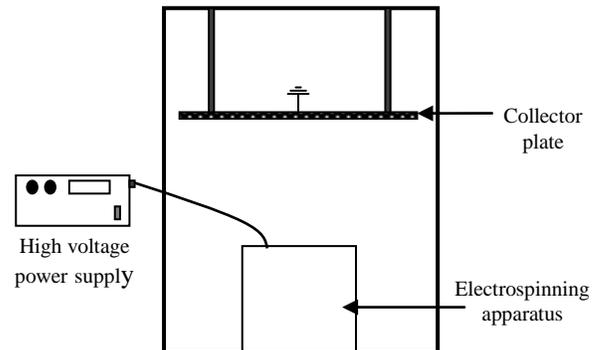
Fig. 4. Schematic drawing of the experimental setup.
