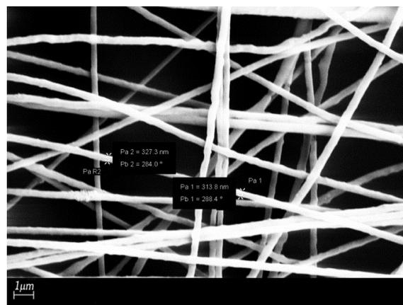
Fig. 5. SEM image of centrifugally electrospun PEO nanofibres.
