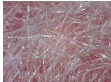
Fig. 1. Photograph of the nonwoven polypropylene media.
