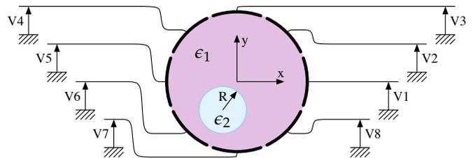
Figure 1. An 8-electrode ECT sensor
