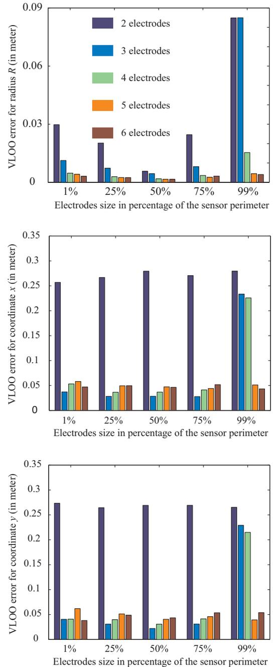
Figure 2. VLOO error for predicting radius  $R$  (top), coordinate  $x$  (middle) and coordinate  $y$  (bottom).
