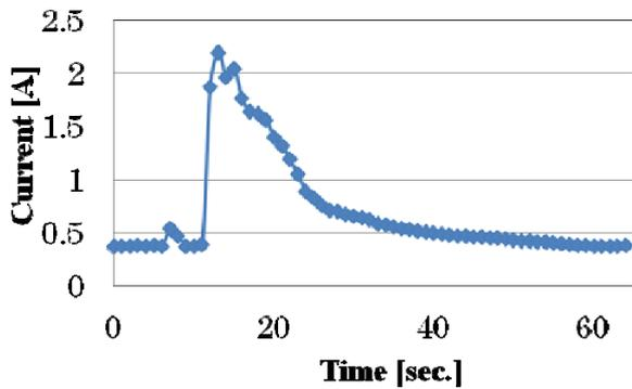
Fig. 8 An electric current of the result for the saline solution of 3.5%, the load of 36 W, and the enhanced plugs when the tracking is generated.
