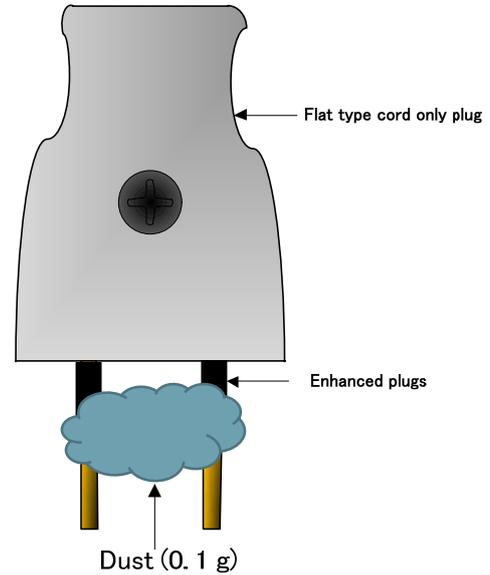
Fig. 3 The dust covered between the outlet and plugs
