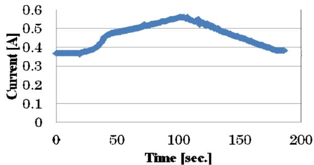
Fig. 4 An electric current of the result for the purified water, the load of 36 W, and a normal plug when the tracking is generated.
