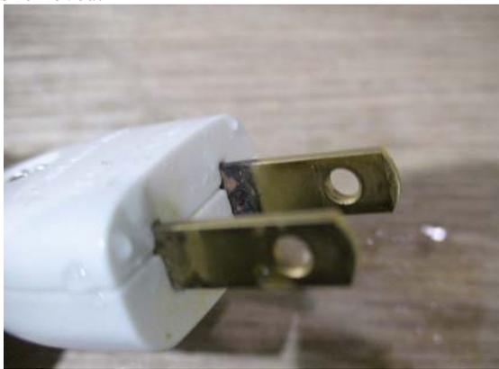
Fig. 5 The photograph of normal plugs at 80 sec. when the saline solution drips.
