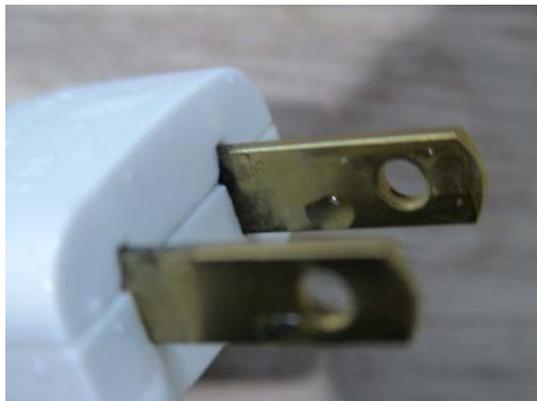
Fig. 7 The photograph of normal plugs at 187 sec. when the purified water drips
