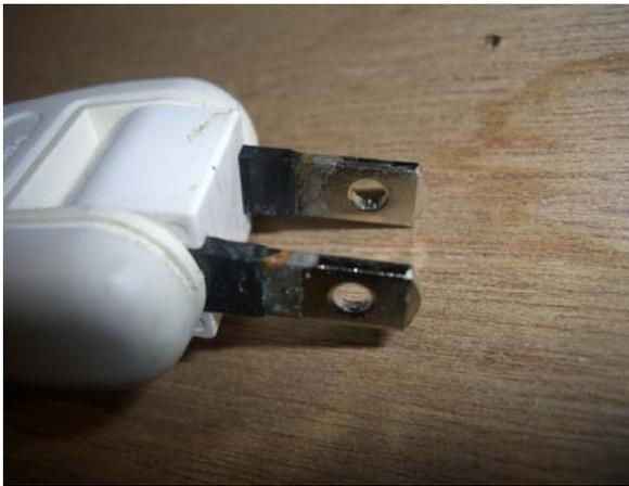
Fig. 9 The photograph of enhanced plugs at 64 sec. when the saline solution drips.
