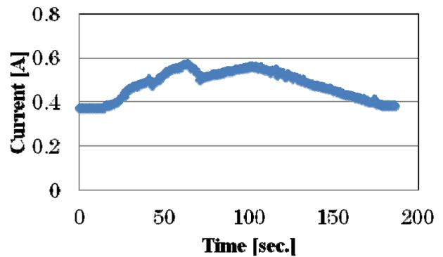
Fig. 10 An electric current of the result for the purified water, the load of 36 W, and the enhanced plugs when the tracking is generated.
