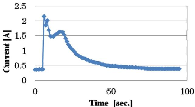
Fig. 4 An electric current of the result for the saline solution of 3.5%, the load of 36 W, and a normal plug when the tracking is generated.
