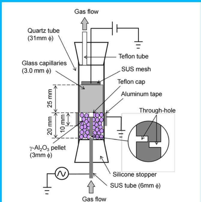
Fig. 3. Schematic illustration of an original honeycomb discharge reactor.
