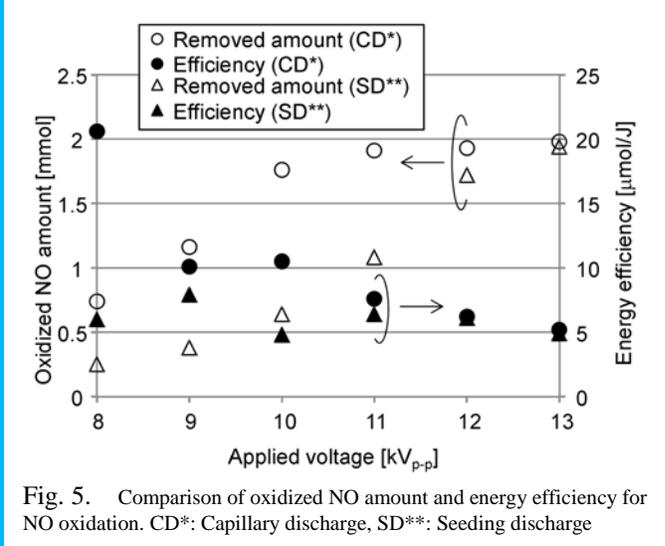
Fig. 5. Comparison of oxidized NO amount and energy efficiency for NO oxidation. CD\*: Capillary discharge, SD\*\*: Seeding discharge
