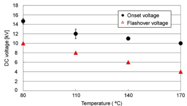
Fig. 9. Influence of temperature on onset and flashover voltage of a capillary discharge when surface discharge was used as a seeding discharge.
