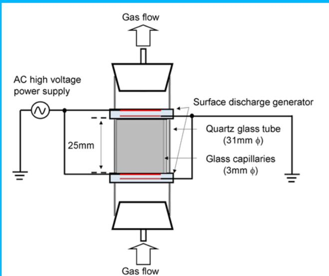
Fig. 1. Schematic illustration of a honeycomb discharge reactor.
