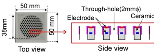
Fig. 2. Schematic illustration of a surface discharge generator.
