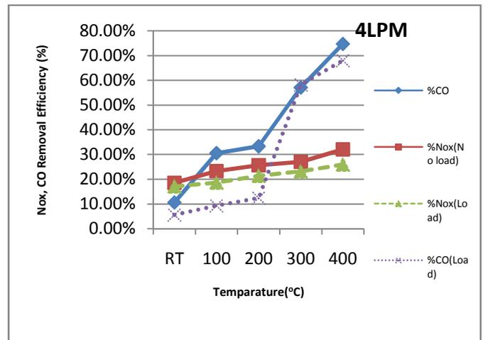
Fig.5. Effect of load on Nox & CO in Red Mud Catalyst removal
