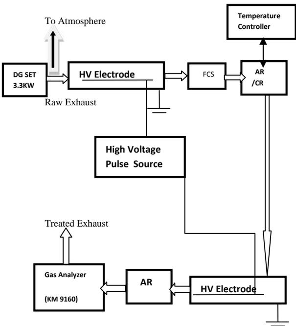
Fig. 1b. Diesel engine exhausts treatment using double step plasma/plasma hybrid technique.
