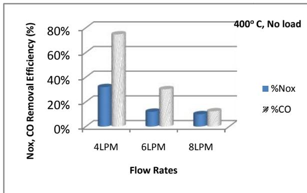
Fig.6 Effect of flow rate on Nox & CO removal in Red Mud Catalyst
