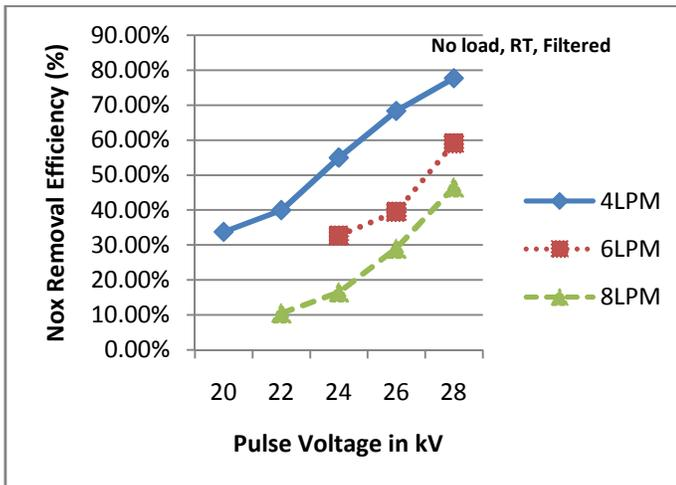
Fig.2. Effect of Flow rate on Single step plasma
