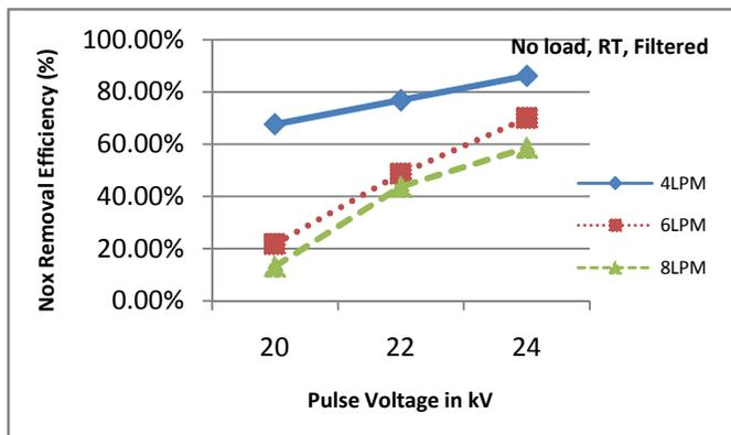
Fig.3. Effect of Flow rate on Double step plasma
