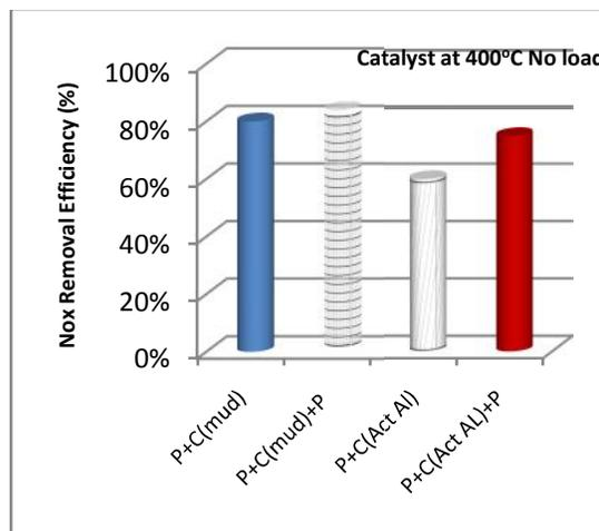
Fig.8. Comparison between single step and double step plasma assisted catalytic process
