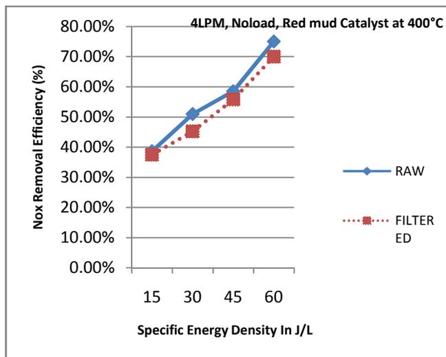
Fig.7.Effect of exhaust nature on single step plasma assisted catalytic process
