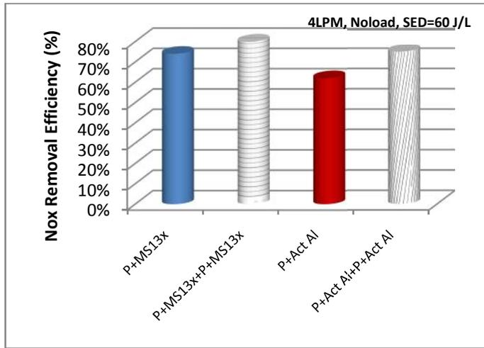
Fig.9 Comparison of single step and double step plasma assisted adsorbent process
