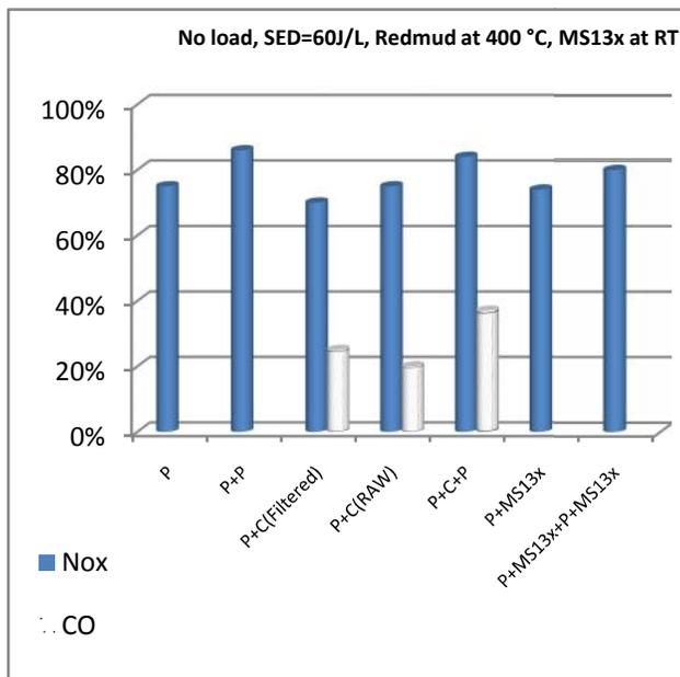
Figure. 10 Performance of different types of techniques for removal of NO<sub>x</sub> & CO
