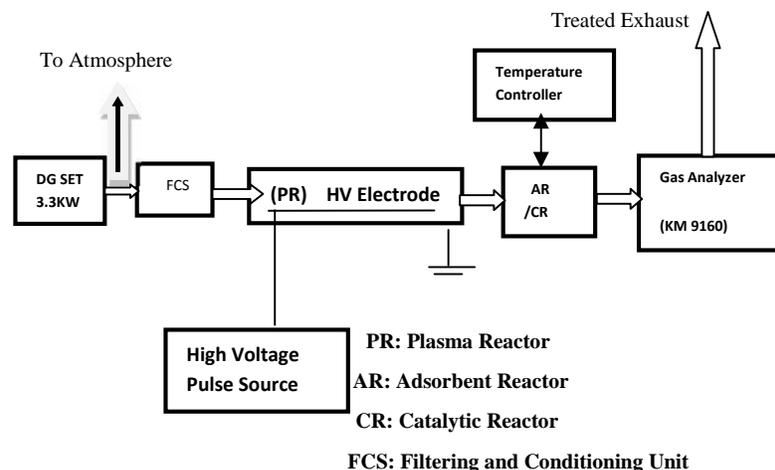
Fig.1a. Diesel engine exhausts treatment using single step plasma/plasma hybrid technique
