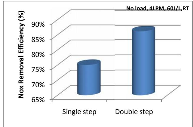
Fig.4. Comparison of single step and double step plasma
