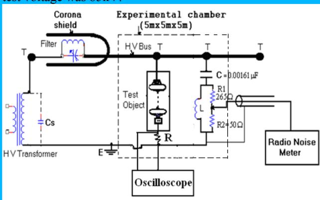
Fig. 1. RIV Measuring circuit as per IEC [2] augmented with ground end current measurement
