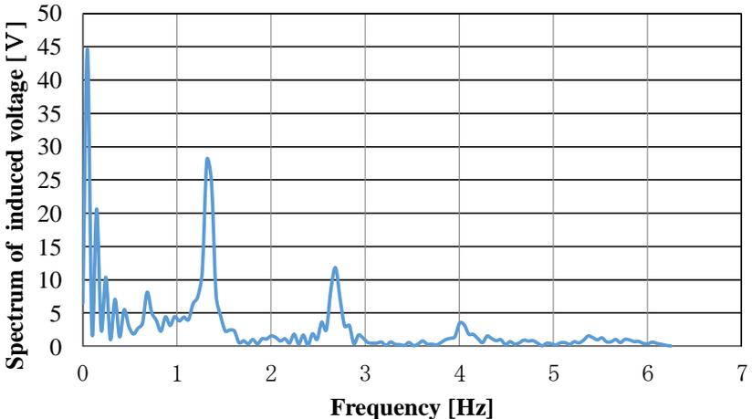
Fig.3. Frequency spectrum of walking motion
