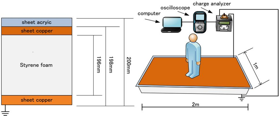
Fig.1. Experiment layout drawing
