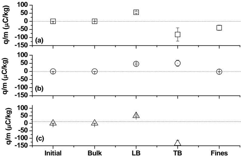
Fig. 5. Results of the net charge-to-mass ratio of the initial, bulk, loosely (LB) and tightly bound (TB), and fine particles. (a) Bubbling flow regime at atmospheric; (b) Turbulent flow regime at atmospheric; (c) Bubbling flow regime at 3 barg.
