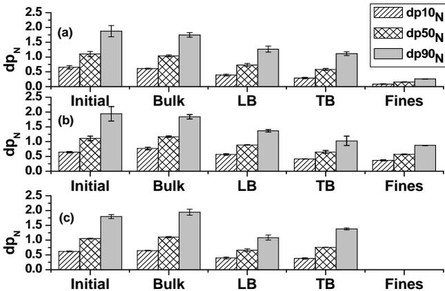
Fig.3. Normalized particle size ( $dp_{10N}$ ,  $dp_{50N}$ ,  $dp_{90N}$ ) in different regions of the fluidized bed. (a) Bubbling flow regime at atmospheric; (b) Turbulent flow regime at atmospheric; (c) Bubbling flow regime at 3 barg.
