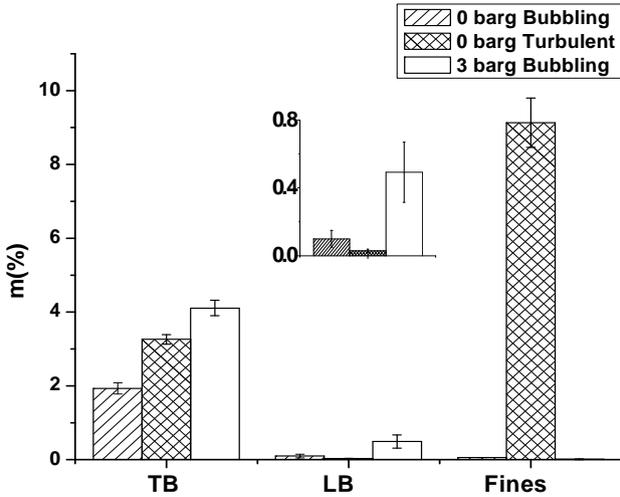
Fig. 2. Results of the mass percentage of particles collected off of the column wall and entrained fines.
