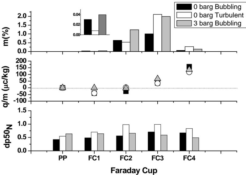
Fig. 6. Results of the charged particle separator of loosely bound particles. PP stands for positive plate.
