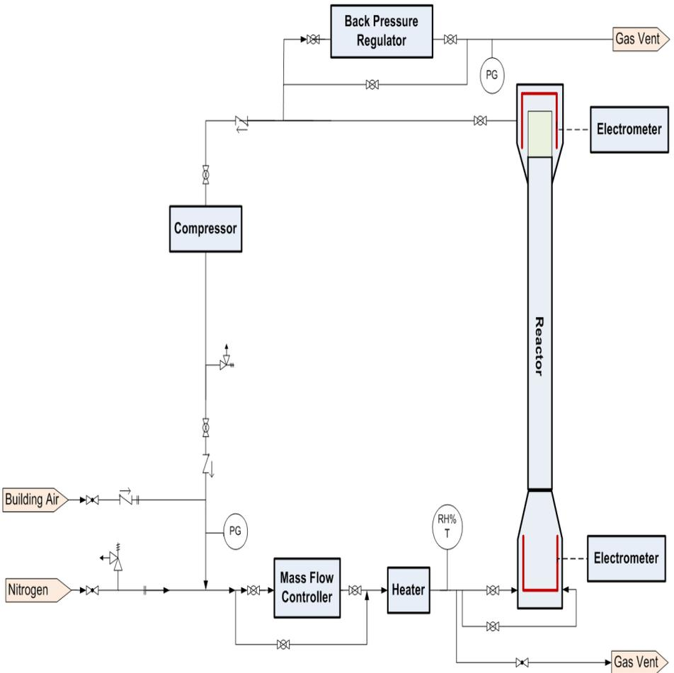
Fig. 1. Schematic diagram of the high-pressure fluidization system.
