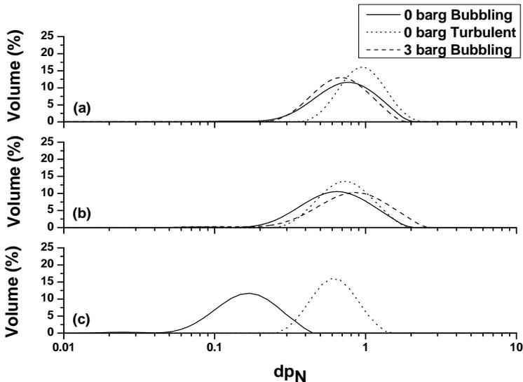
Fig. 4. Normalized particle size distribution. (a) Loosely bound; (b) Tightly bound; (c) Fine particles.
