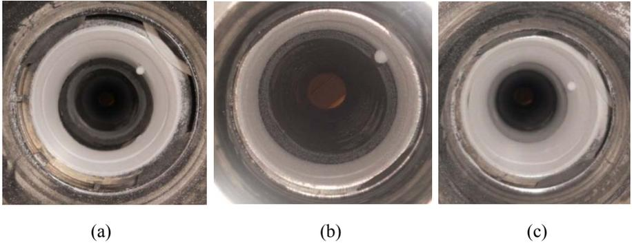
Fig.7. Images of wall fouling. (a) Bubbling flow regime in atmospheric; (b) Turbulent flow regime in atmospheric; (c) Bubbling flow regime at 3 barg.
