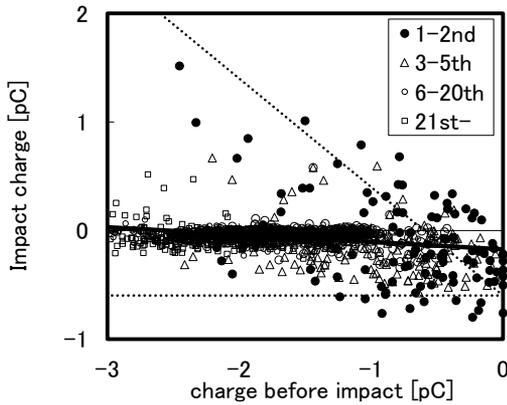
Fig. 4. The relationship between the impact and charge before impact, which integrates the many results of single particles of 200  $\mu\text{m}$ .
