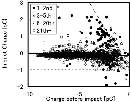
Fig. 3. The relationship between the impact and charge before impact, which integrates the many results of single particles of 300  $\mu\text{m}$ .
