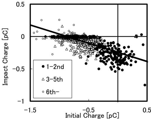
Fig. 5. The relationship between the impact and charge before impact, which integrates the many results of single particles of 100  $\mu\text{m}$ .
