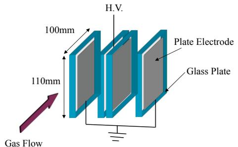
Fig.3. Electrode configuration of the DBD type ESP.
