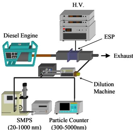
Fig.2. Schematic diagram of the experimental setup for DBD type ESP.
