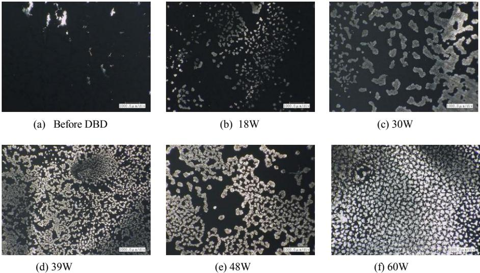
Figs.7. The picture of the electrode surface after 20min DBD operation loads.
