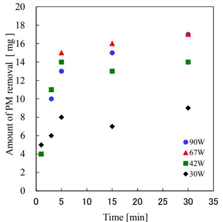
Fig. 6. Time-dependent the amount of PM removal as a function of the discharge power.
