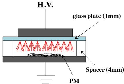
Fig.1. Dielectric barrier discharge reactor.
