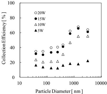
Fig. 8. Particle-size dependent collection efficiency as a function of the discharge power of 5-20 W.
