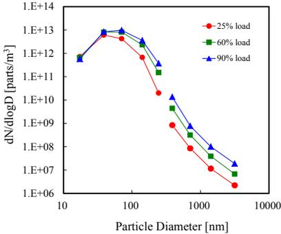
Fig. 4. The particle-size dependent number density from the diesel engine particulates.
