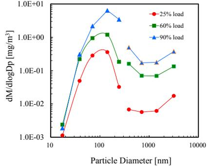
Fig. 5. Particle-size dependent mass-base density from the diesel engine particulates.
