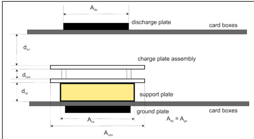
Fig 3. Shielding measurement assembly in a card box
