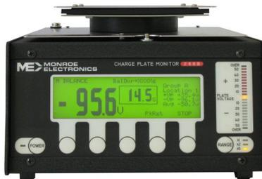
Figure 3. A typical commercial charge plate monitor.
