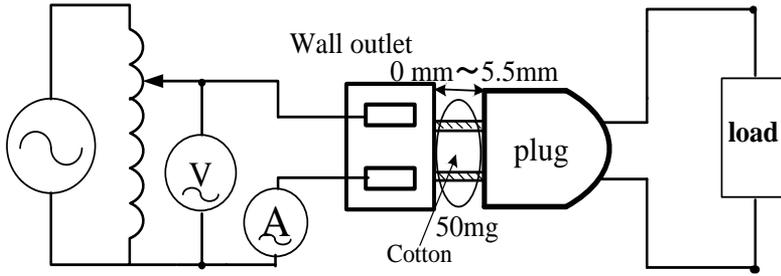
Fig.1 experimental circuit
