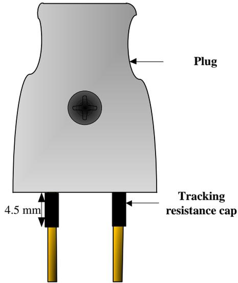
Fig.2 Tracking resistance plug
