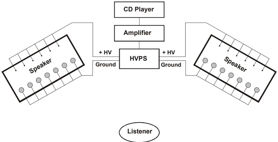
**Fig. 1.** Schematic representation of Kronos acoustic system that uses two Kronos EFA loudspeakers.
