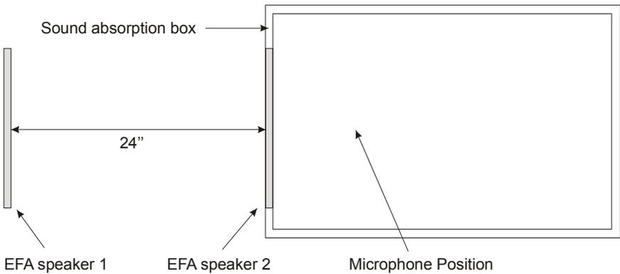
**Fig. 5.** Experimental setup for active noise cancellation tests.
