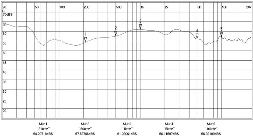
**Fig. 3.** Frequency response of Kronos EFA loudspeaker.
