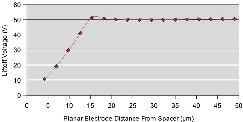
**Fig. 4: Liftoff voltage as a function distance from left side electrode of the cell in Fig. 1 for 2.8 μm diameter particles charged to 30% of maximum ( $f_{\text{real}} = 0.3$ ). Only data from the left half of the cell is shown as the right half is the mirror image.**
