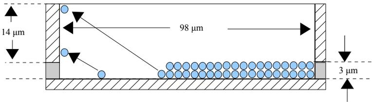
**Fig. 1: Diagram showing a cell of the ESPD device under analysis**
