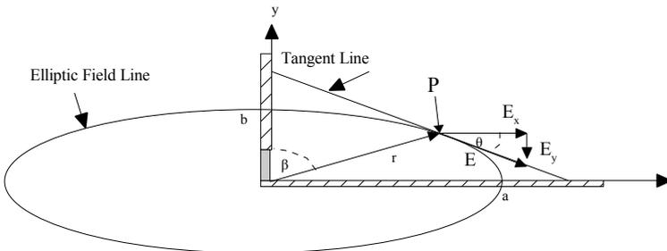
**Fig. 3: An elliptical field line located in the  $xy$  has a particle at point  $P$  on this line a distance  $r$  from the origin. The angle  $\theta$  is between the tangent Line and the  $x$ -axis, whereas, the angle  $\beta$  is between  $r$  and the  $y$ -axis.**
