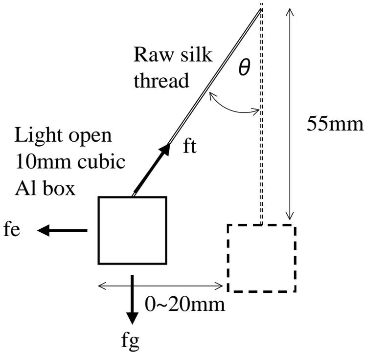
Fig. 11. Schematic diagram of the first and second position of the right open cubic Al box. At first, the cubic Al box is hanged by a raw silk thread (a dotted line), then the box is moved to left by the asymmetric force (a solid line). “ $f_g$ ”, “ $f_e$ ” and “ $f_t$ ” are the gravity force, the electric (asymmetric) force and the tension of the thread respectively. “ $\theta$ ” is the angle between the first and second position of the thread. .
