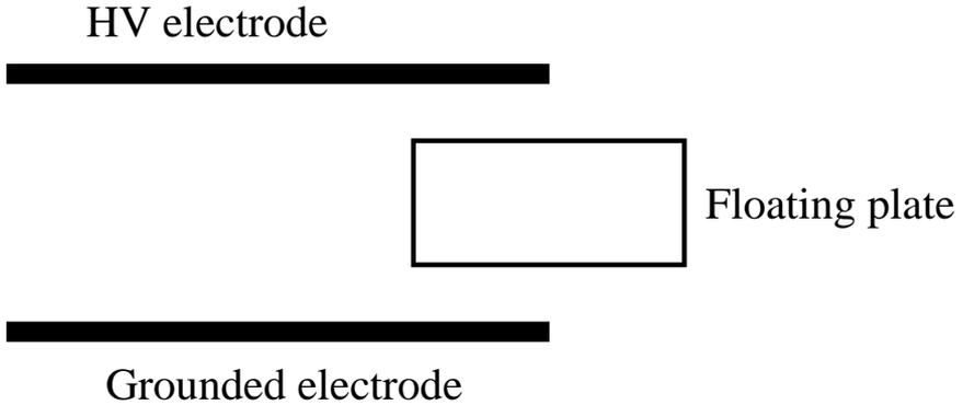
Fig. 1. Freshmen's problem. A floating metal plate which has no charge is inserted by half between electrodes. The upper electrode is applied high voltage and the lower electrode is grounded.
