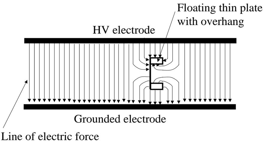
Fig. 6. Lines of electric force around the floating thin plate with overhangs which is placed center between the high voltage applied upper electrode and the grounded lower elec-
