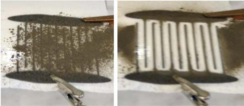
Fig. 9. Before and after photographs of a dust shield on fabric with JSC-1A lunar simulant.
