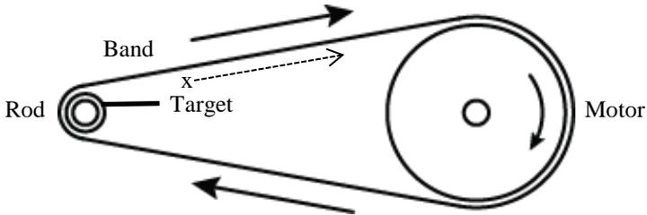
Fig 1: A diagram of the apparatus used to produce x-rays from a tribocharged insulating band. The band is constructed of insulating polymer. It is run over a stationary metallic rod. A small metal target is placed near the rod and below the insulating band. The band is moved around the stationary rod via a motor at 1000-10,000 rpm while the system is held at a pressure below  $10^{-4}$  torr.
