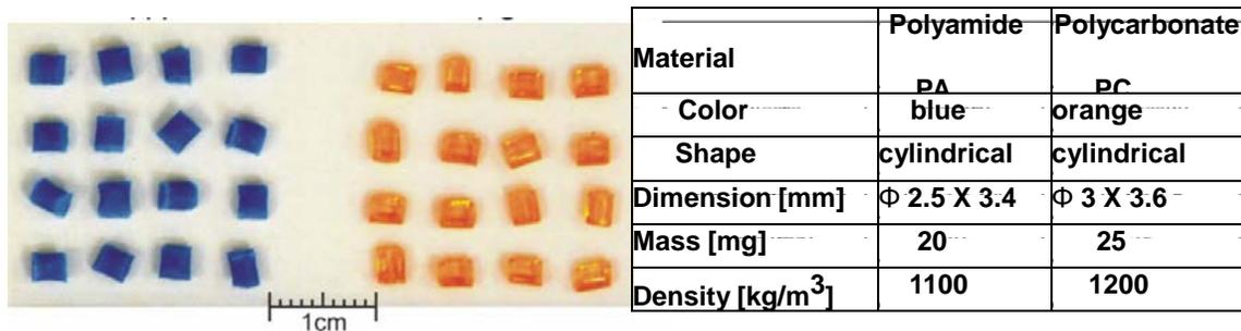
Fig. 6. Aspect (a) and characteristics (b) of PA and PC granules used in tribo-aero-electrostatic separation.
