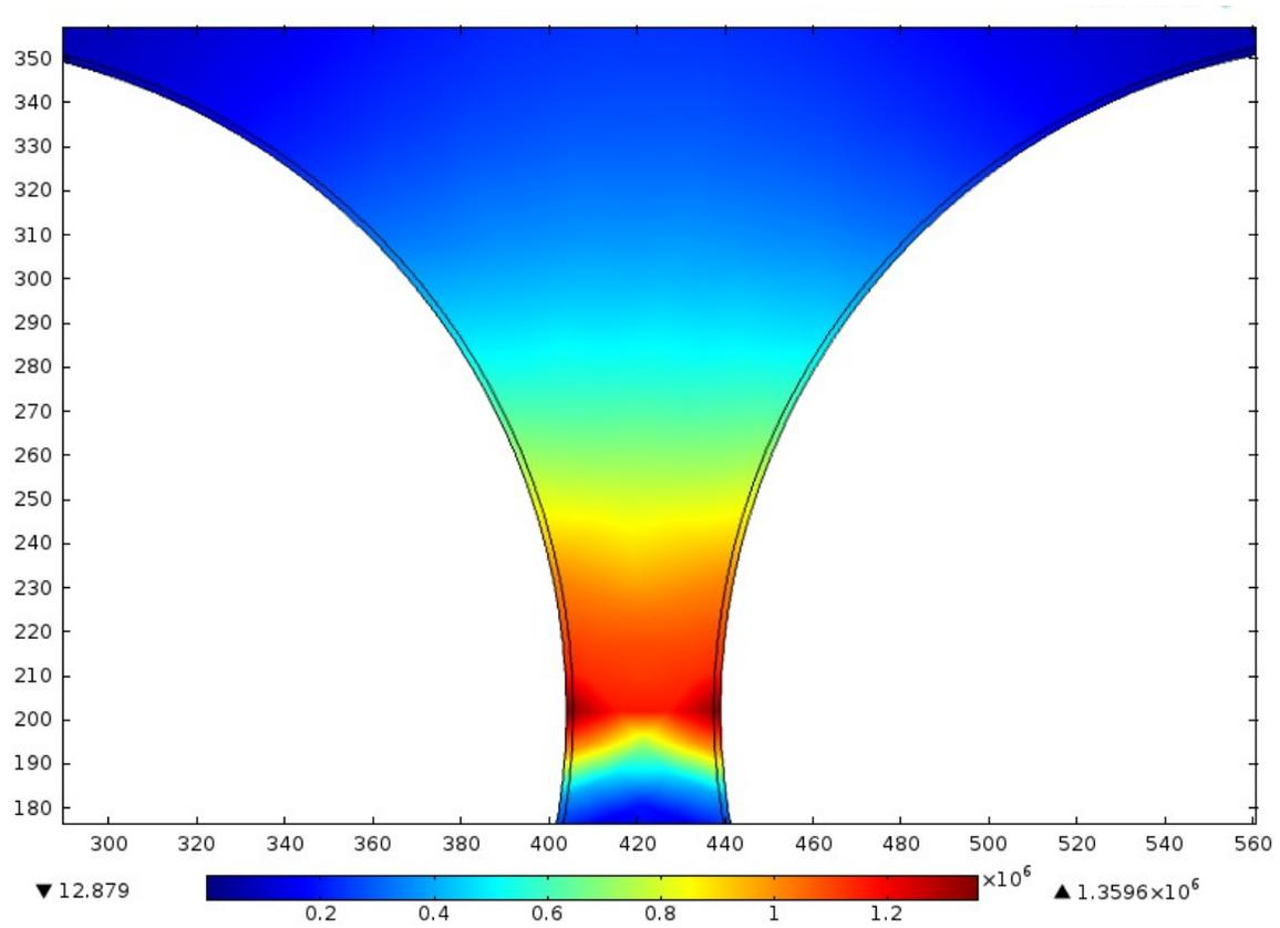
Fig. 4. Electric field distribution between the high voltage electrodes of the novel tribo-aero-electrostatic separator, supplied at  $\pm 20$  kV.
