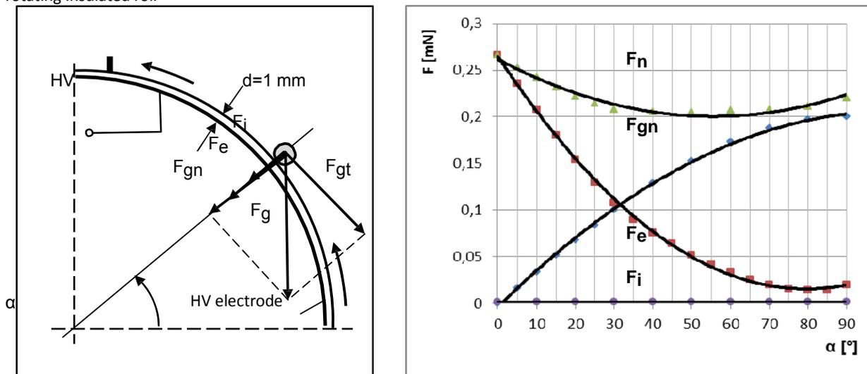
Fig. 5. Forces acting on a charged granule pinned on the surface of the insulated roll (a) and evolution of the pinning forces versus granule position  $\alpha$  (b). The granule mass was considered 20 mg and the charge 0.2 nC. The electric field strength was calculated for  $\pm 20$  kV high voltage level.
