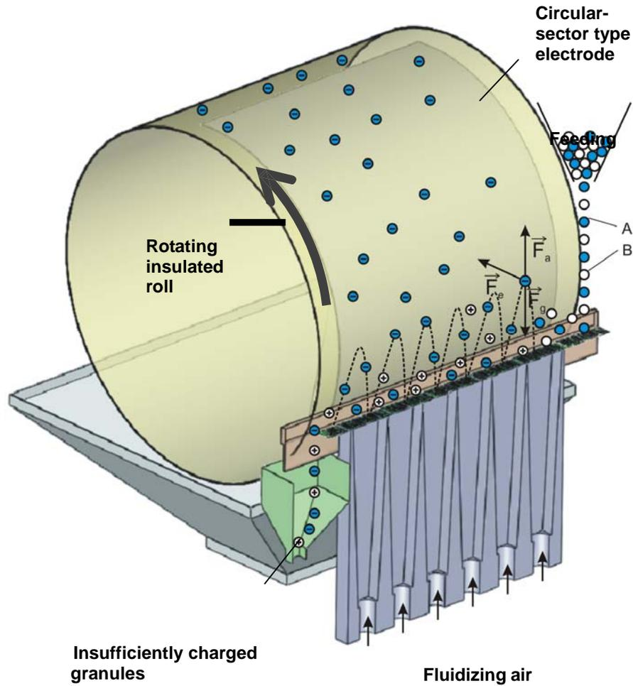
Fig. 2. Charging and separation process in the novel tribo-aero-electrostatic separator.
