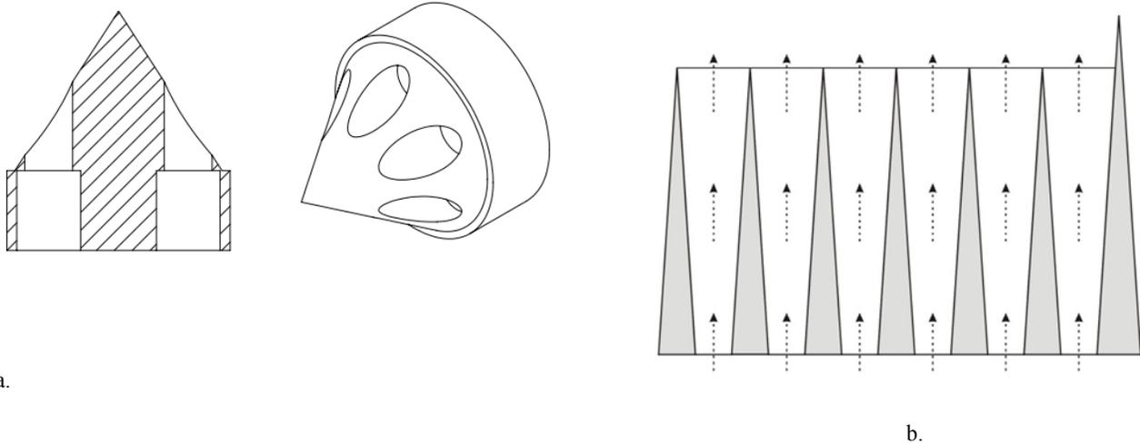
Fig. 3. Divider of the turbo-blower air flow (a) and the six compartments air chamber of the separator (b).
