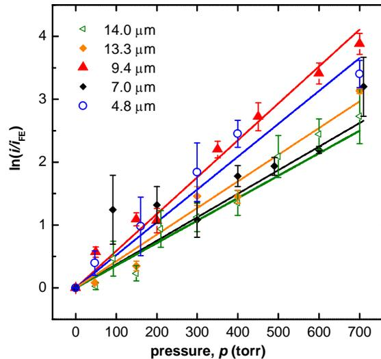
Fig. 1 Logarithmic plot of normalized current as a function of pressure  $p$  for electrode gaps of 14.0, 13.3, 9.4, 7.0 and 4.8  $\mu\text{m}$  operating at 350 V and using laboratory air.
