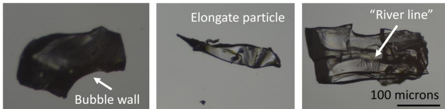
Fig. 5: Particles from a fragmentation event displaying morphological similarities to real ash particles [15].
