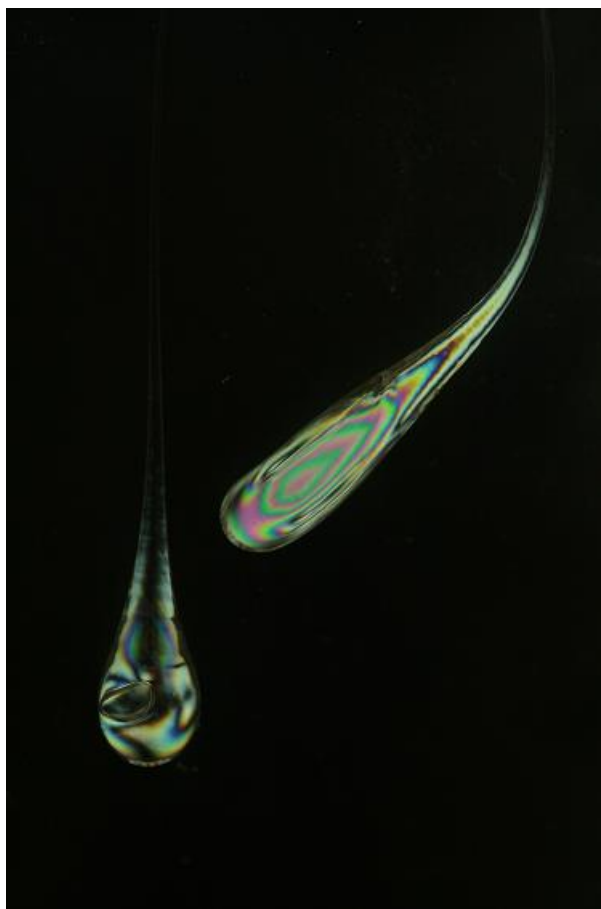
Fig 1: Two Prince Rupert's drops under polarized light. Notice the stress patters. Left drop includes a bubble.
