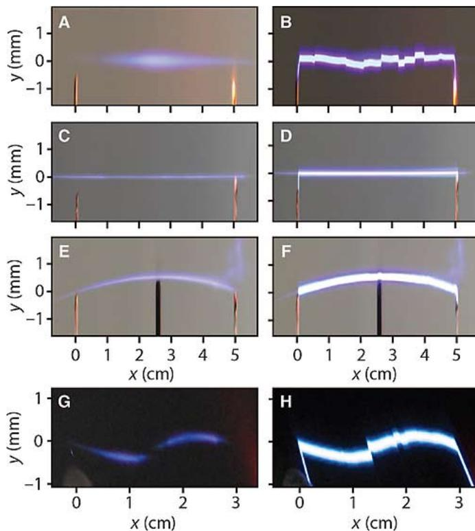
Different shapes of discharge achieved based on the type of beam used. A and B: Gaussian beam (control). C and D: Bessel beam. E and F: Airy beam. G and H: S-shaped beam obtained by combining two conventional Airy beams. Left: Photographs taken when no voltage is applied (only the laser beam is visible). Right: Discharge in the presence of high voltage between the two electrodes.
