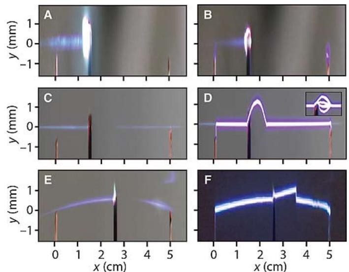
A and B: Gaussian beam (control). C and D: Bessel beam. E and F: Airy beam. Left: Laser beam with no voltage applied in the presence of an obstacle. Right: For both the Bessel and Airy beams, the discharge follows the laser and circumvents the obstacle before reconstructing itself. The inset in D is a multi-shot photo of the various trajectories the discharge take around the obstacle before converging on a single rectilinear trajectory.
