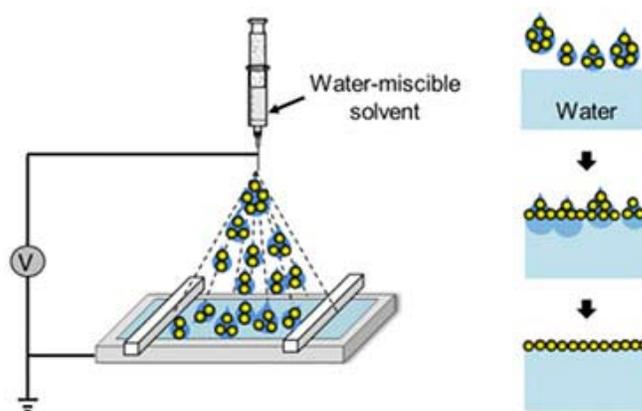
Using an electro spray can spread a water-soluble solvent with nanoparticles onto water's surface without mixing.
