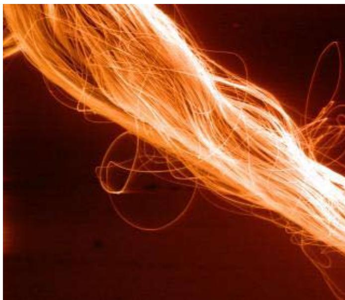
High-resolution scanning electron microscopy shows a portion of a large bundle of ultra-strong and tough continuous nanofibers developed by UNL researchers. (Photo: Joel Brehm, Dimitry Papkov, Yuris Dzenis)
