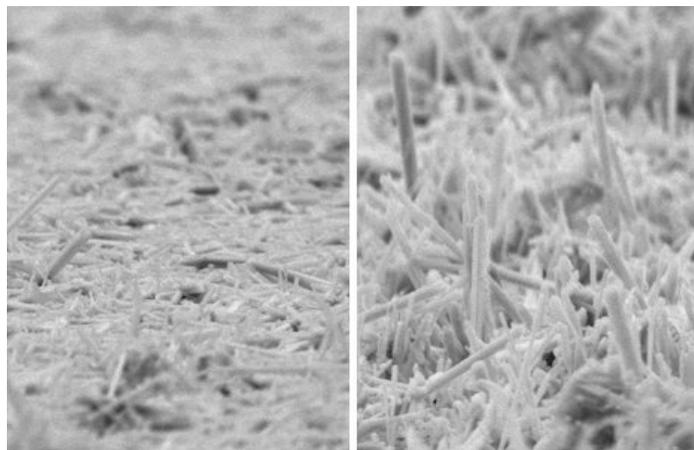
The non-aligned manganese dioxide nanorods on the left were made using conventional methods. The aligned nanorods on the right were grown in Dennis Desheng Meng's lab using electrophoretic deposition. Photos by Sunand Santhanagopalan
